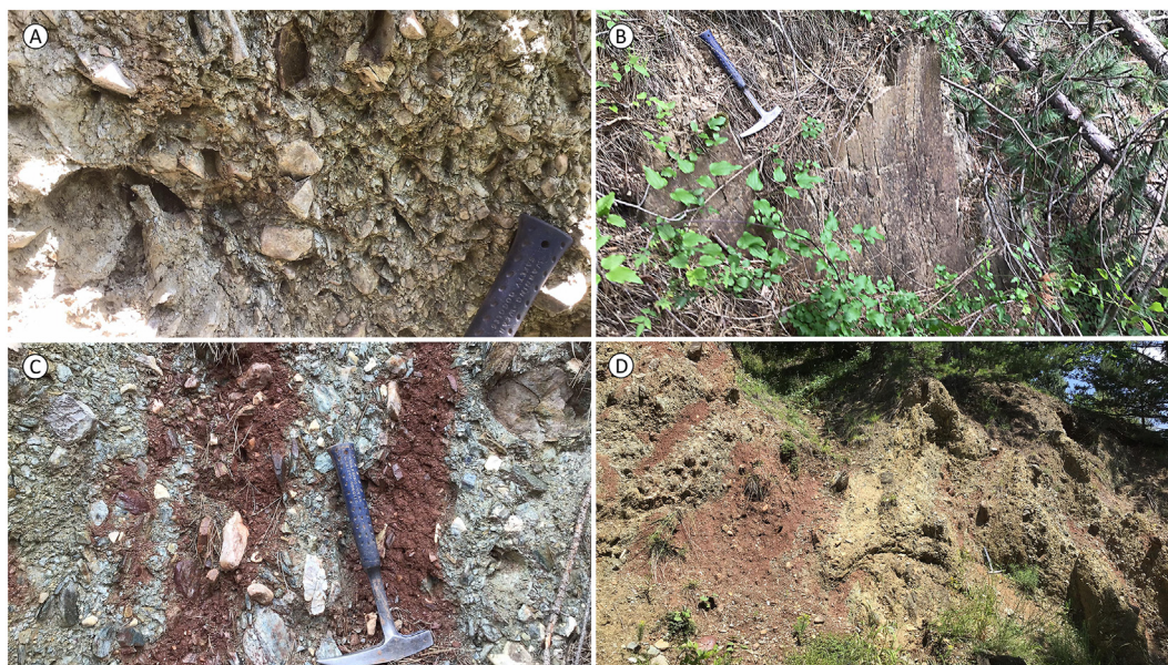
Fig. 18. Appearance of the main boundary fault and the associated damage zone in the field: calcareous cemented fault breccia – L55 (A); fault scarp with 180/82 azimuth and dip (B); cataclastic red clayey zones formed in the proximal alluvial fan deposits (C); shear zones (red) and drag fold in the proximal alluvial fan deposits – L66 (D).
