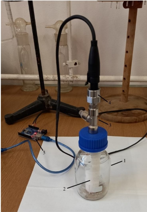
Fig. 2 Calcimeter composition: (1) glass container with lid, (2) cylindrical plastic tube, (3) metal reduction with purge valve, (4) pressure sensor, (5) Arduino board.
