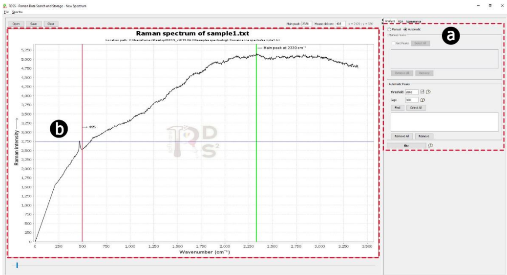
Fig. 4 Automatic peak finder operation used on a high-fluorescence Raman spectrum by setting the threshold (b) and gap variables.
