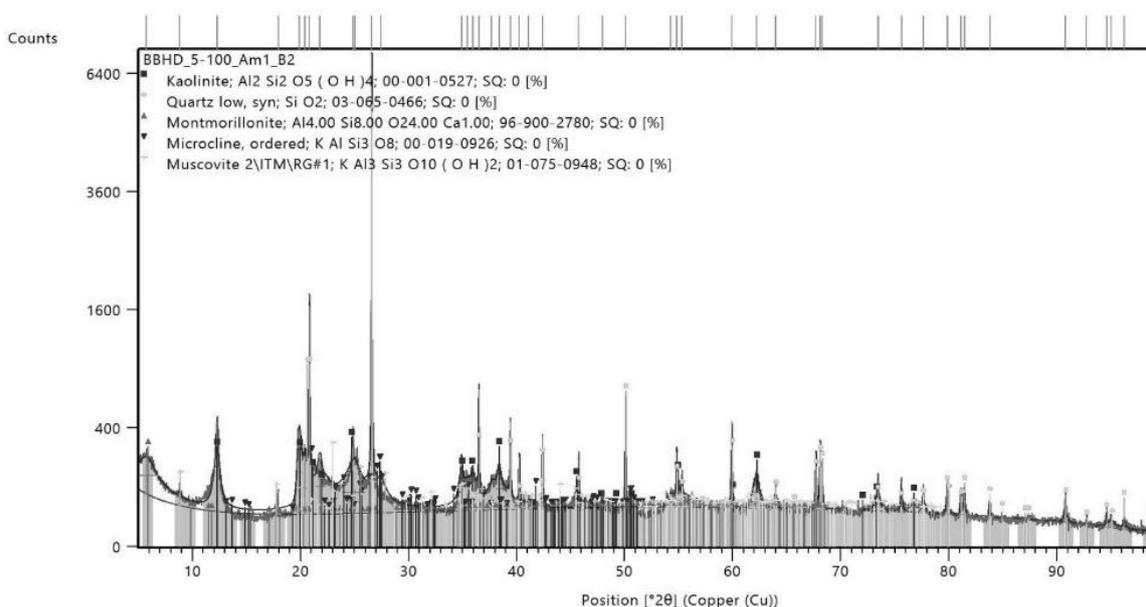
Fig. 10. XRD result of reject sample 2 (AM-01/B2).
