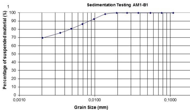
Fig. 7. Grain size distribution curves of sample AM1-B1.
