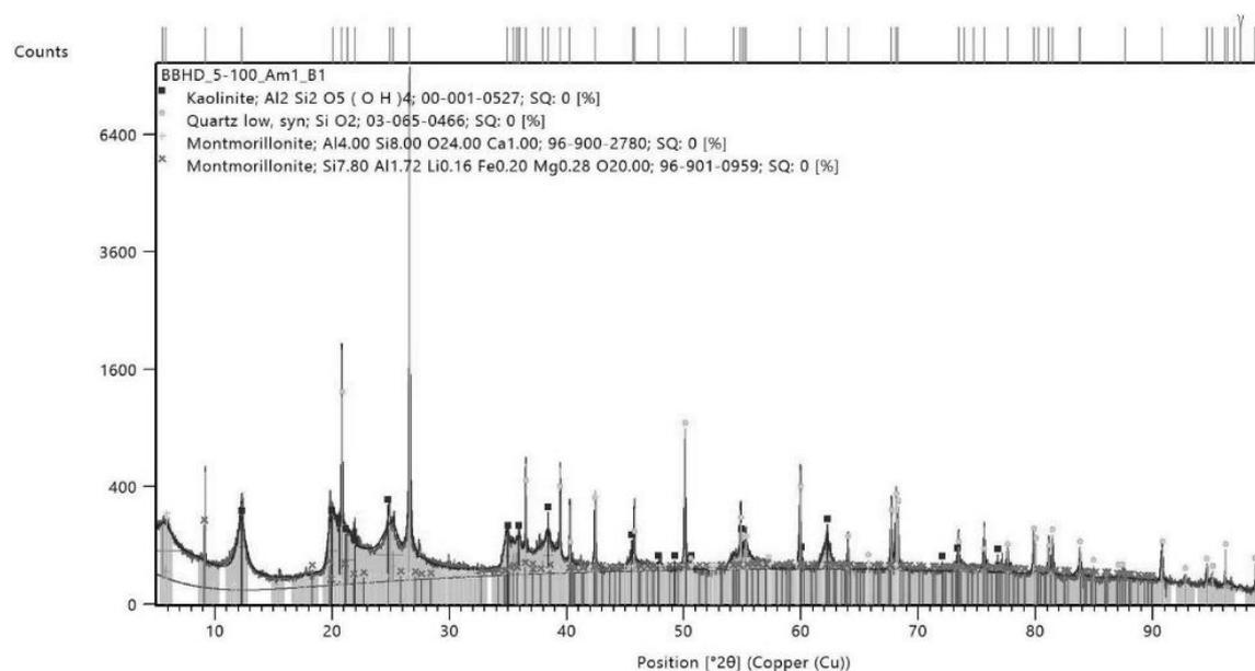
Fig. 9. XRD result of reject sample 2 (AM-01/B1).
