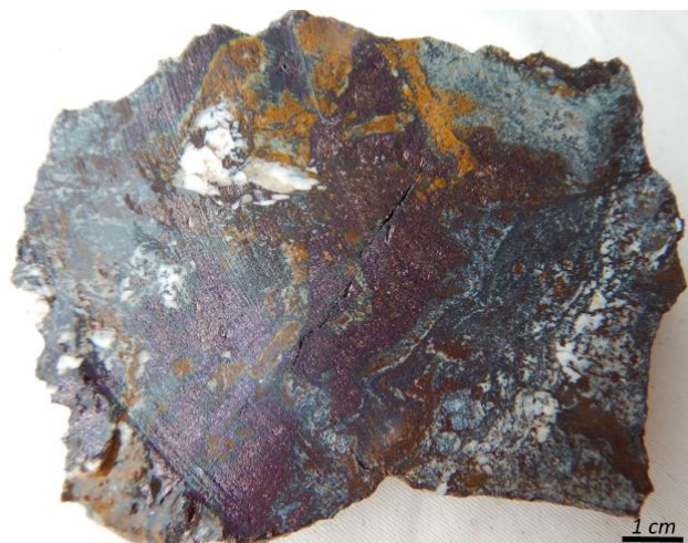
Fig. 2. Slice of the ore sample from Blidar Contact ore body used for geochemical analyses. Bornite (dark purple) is the main ore mineral and is associated to wollastonite (white).
