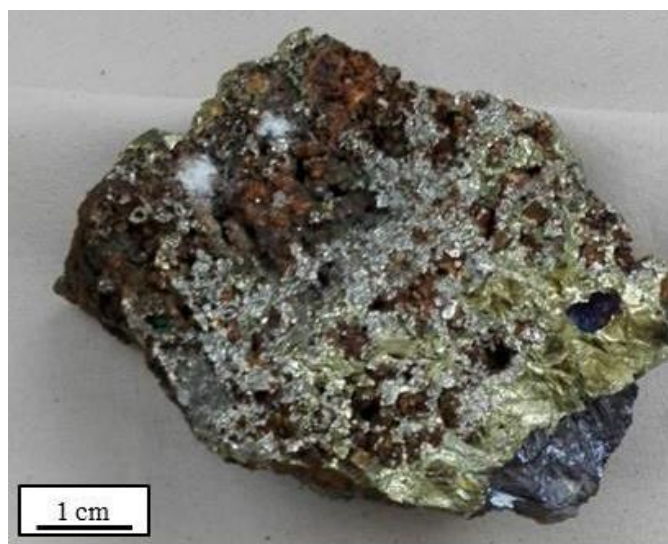
Fig.2. The studied ore sample BT5089 from Cisma, used for geochemical analyses, dominated by pyrite and chalcopyrite.
