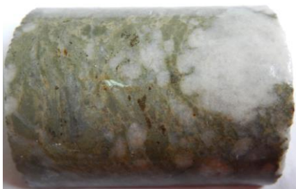
Fig. 1. Matrix-supported conglomerate with carbonate pebbles; dimensions of the sample: 6.5 x 5.5 cm.
