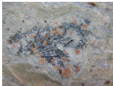
Fig. 2. A nest composed of remnant calcite, black needle-like crystals, light brown isometric crystals and pyrite; approx. dimensions of the field view: 4 x 3 cm.
