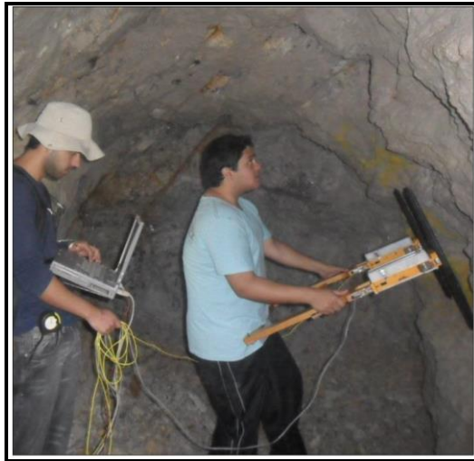
Fig. 2: Photo of the acquisition of GPR profile on the wall of the pegmatite rock.
