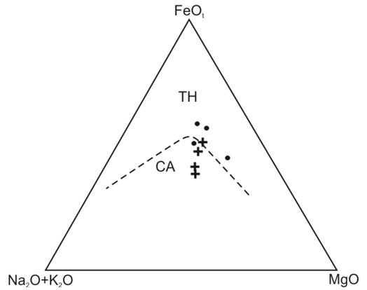
Fig. 2 Plotting of the average values of the rocks from the two basalt series in the  $\text{FeO}_{\text{tot}}-(\text{Na}_2\text{O}+\text{K}_2\text{O})-\text{MgO}$  diagram. Fields according to Irvine and Baragar (1977). Data from Tables 1 and 2. Legend as in Figure 1.
