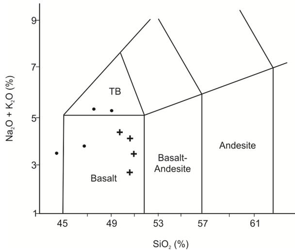
Fig.1. Plotting of the average values of basalts and related rocks from the two rock series on the Na<sub>2</sub>O + K<sub>2</sub>O vs. SiO<sub>2</sub> diagram. Fields according to Le Bass et al. (1986). Dot – pre-ocean basalts; cross – post-collision basalts. Data from Tables 1 and 2.
