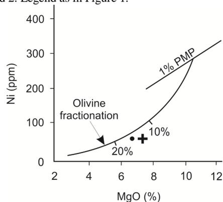
Fig. 10 Plotting of the general average of the rocks from the two volcanic rock series on the Ni vs MgO diagram. Partial melting line (PMP) of 1% pyroxene and olivine fractionation curve according to Volker et al. (1992). Data from Tables 1 and 2. Legend as in Figure 1.
